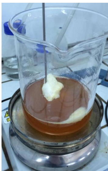
Figure 7. Vegetable oil mixing with NaOH/Methanol solution
