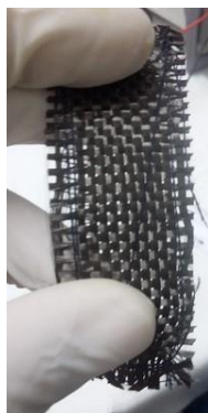
Figure 2 – Flexible carbon fiber electrode.
