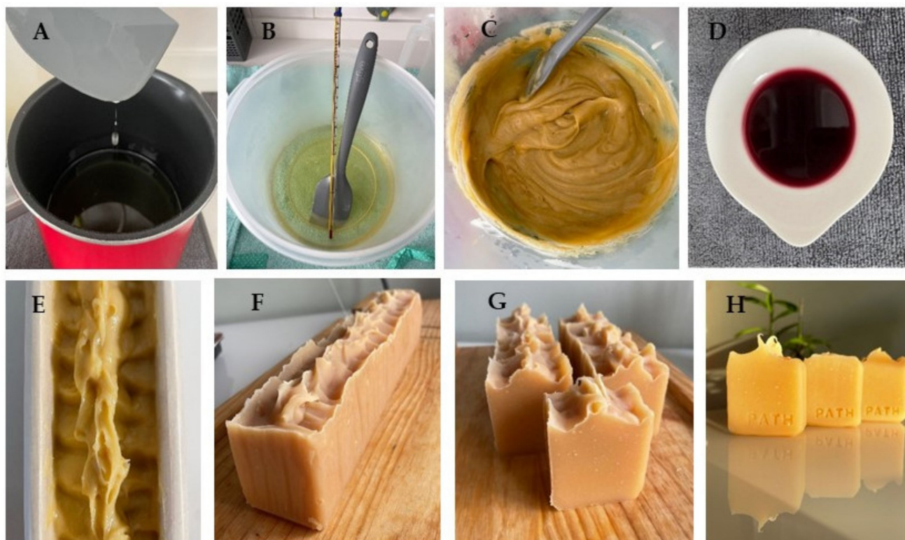
Figure 4. Juçara natural soap production. (A) Oil and butter heating; (B) melted butter and oil mixture; (C) soap mass before additives; (D) juçara extract (42.6% of 1,2-propanediol in 1:50 g/mL of juçara dried pulp); (E) parchment paper-lined molds filled with soap mass; (F) loaf of soap after 24 h; (G) soap bars; and (H) soap bars after cure.
