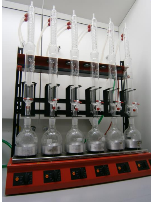
Figure 7 Soxhlet apparatus used in the extraction of crude fat.
