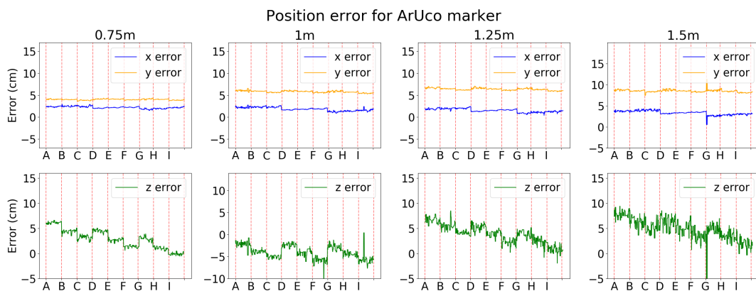
Figure 3.8: ArUco position measurement error per marker position (Table 3.2).
