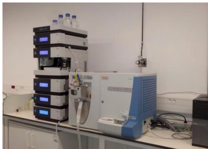
Figure 3 6. HPLC system used for analysis of aloin isomers A and B in Aloe vera and in the final product.
