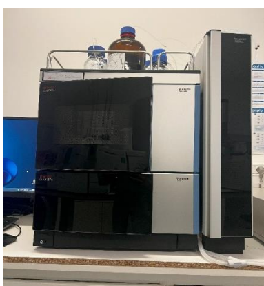
Figure 3. 5. HPLC system used for analysis of fructose and glucose in honey.
