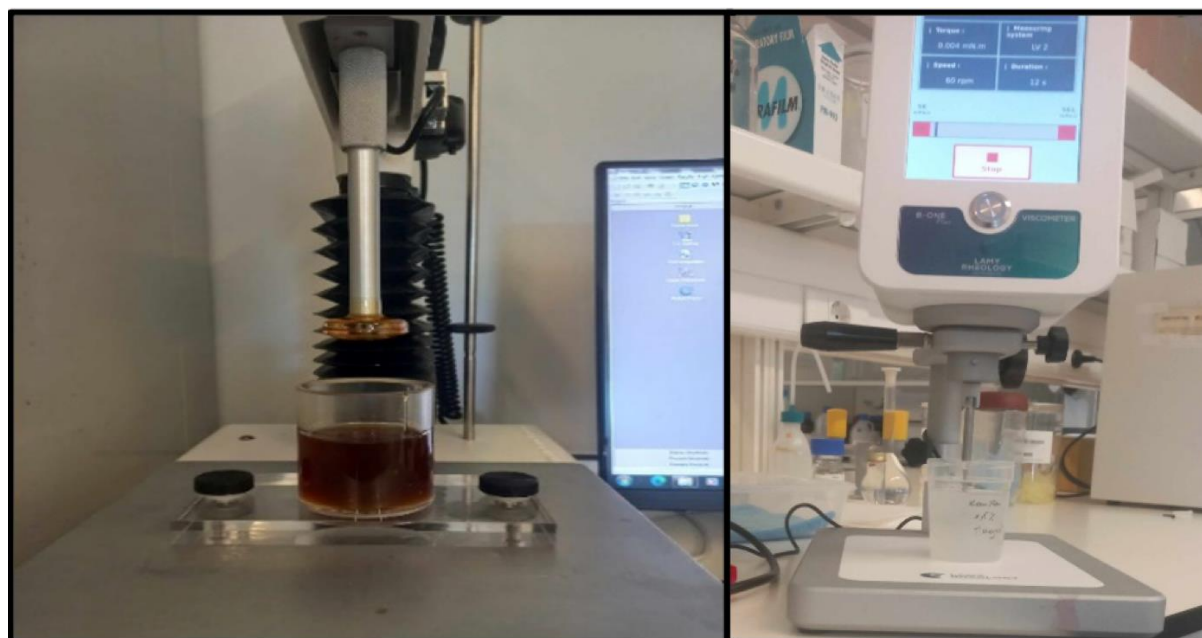
Figure 3.2. Apparatus used for rheological analysis: (left) TA.XT Plus Texture Analyzer for texture measurements and (right) B-One Plus Viscometer for viscosity measurements.
