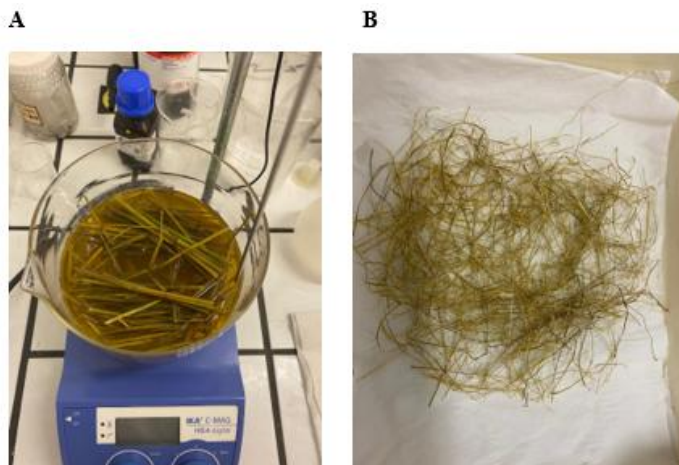
Figure 17-A-Chemical process with the fibers; B-Fibers after the chemical process, ready for drying
