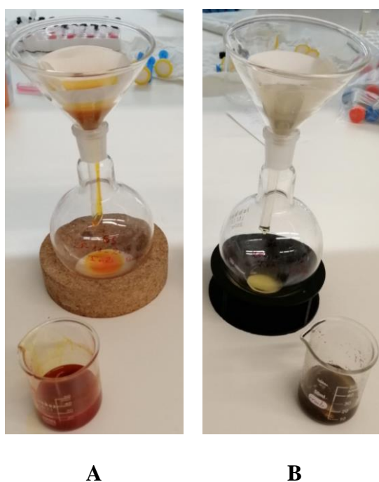
Figure 11. Hydroethanolic extraction from the seeds ( A ) and pods ( B ) of B. orellana .
