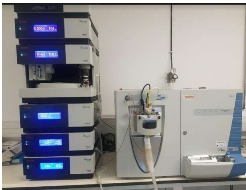
Figure 6 The UPLC–MS/MS instrument
