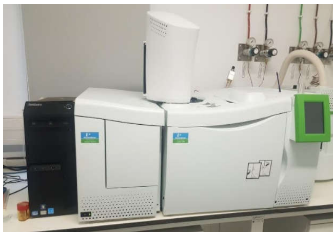
Figure 5: Gas-chromatography coupled with mass spectrometry (GC-MS)
