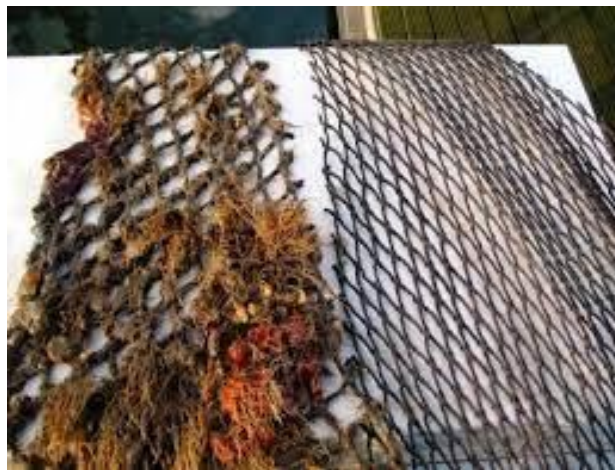
Figure 11 - Demonstration of nets with and without fouling on it.
