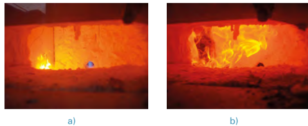
Figure 3. Photograph from inside the furnace. (a) Ignition of the exposed cork board at minute 20. (b) Ignition of the cork unexposed board at minute 36.
