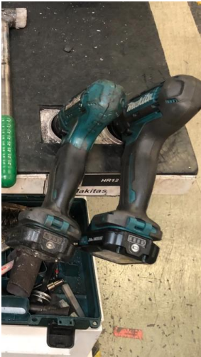
Figure 5.25: Solution implemented for operator 5: Creation of supports on tables to put the screwdrivers
