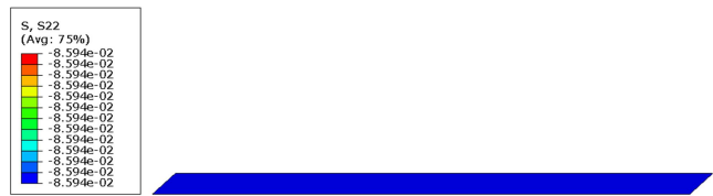
Fig. 8. Normal stress [MPa] in X 2 direction for a applied load of 290 N.
