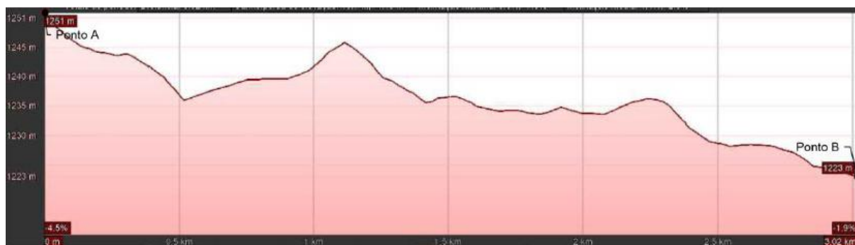
Figure 24. Longitudinal profile of the road
