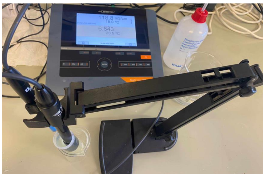
Figure III.4: Multimeter used for pH and conductivity measurements.
