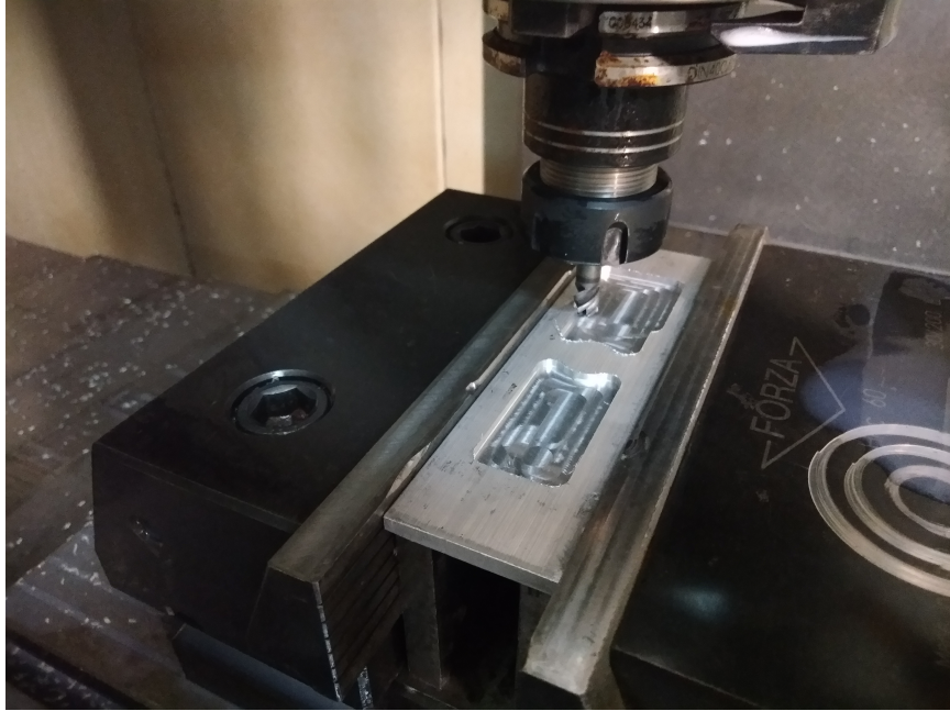
Figure 3.2: Mold being made in a CNC machine.
