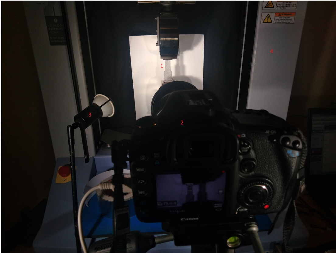
Figure 3.7: Specimen in the Tensile Test for image acquisition indicating: 1 - Specimen; 2 - Camera; 3 - Lightning System; 4 - Universal Test Machine.
