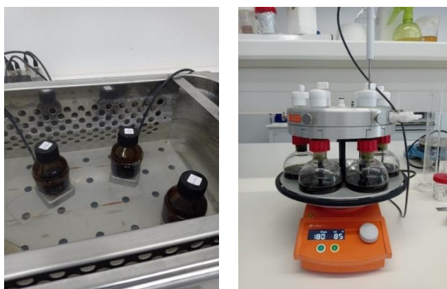
Figure 3.6: HAE extraction of E. globulus leaves performed in a hot water bath (left) and a Carousel 6 Reaction Station coupled with a hot stirring plate (right).
