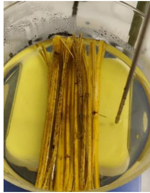
Figure 7 - Hemp Date 1 2 g/l NaOH + 2 g/l NaCO 3 30 minutes.
