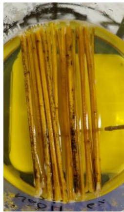
Figure 8 - Hemp Date 4 6% NaOH 30 minutes.
