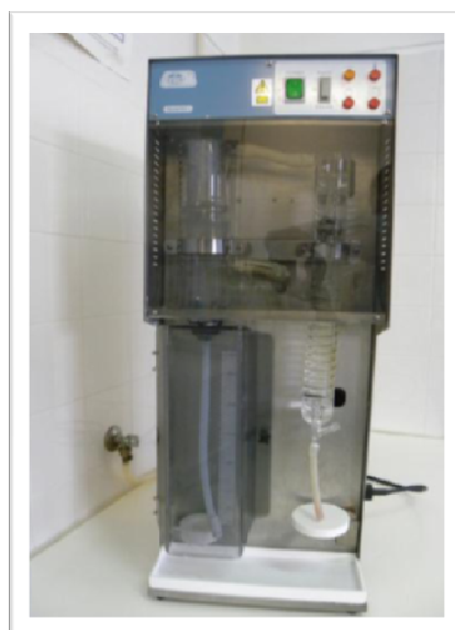
Figure 3.6 - Kjeldahl distiller used in this work to determine total protein of commercial mannoproteins
