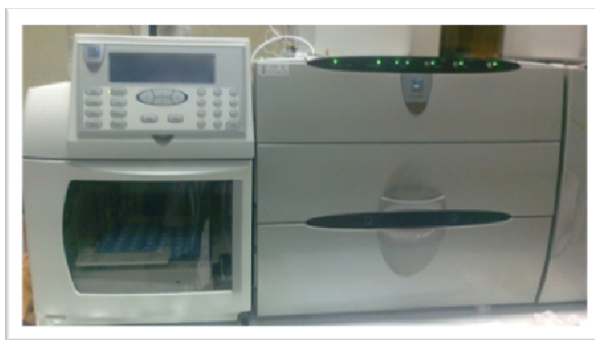
Figure 3.5 - Dionex ICS 3000 used in this work to quantify sugar from commercial mannoprotein
