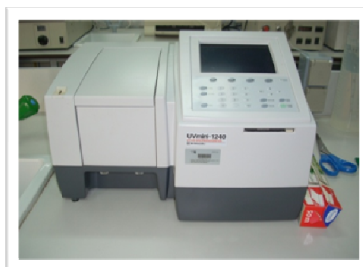
Figure 3.8 - Shimadzu UVmini-1240 Spectrophotometer used in this work
