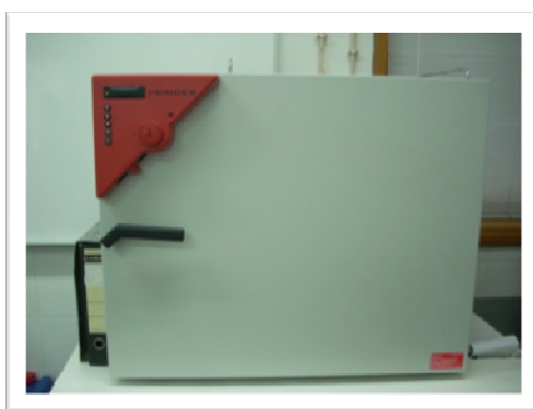
Figure 3.9 - Oven used in this work for browning potential determination
