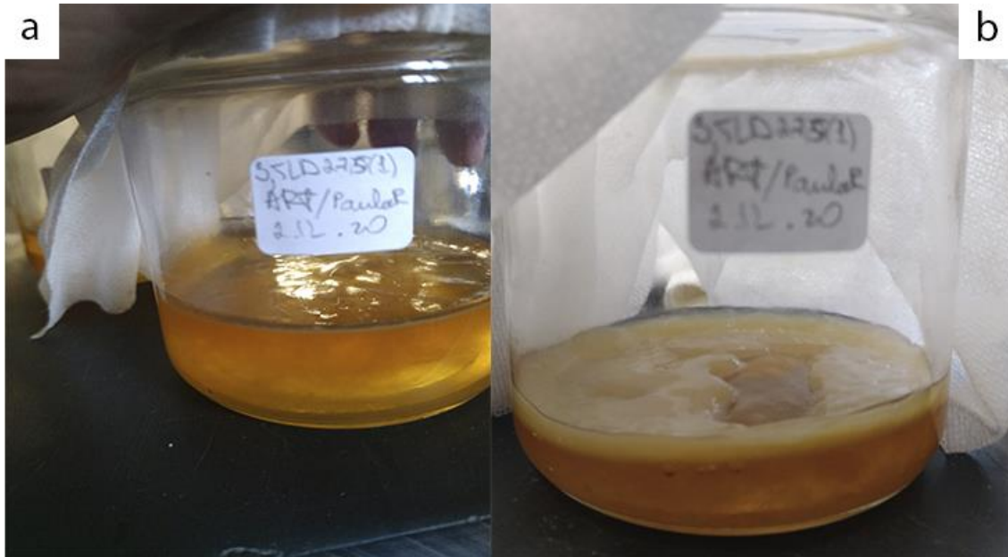
Figure 15 – Formation of cellulose after four days (a), and after 10 days (b) of fermentation at 27.5 °C using 3.5 g/L of black tea.
