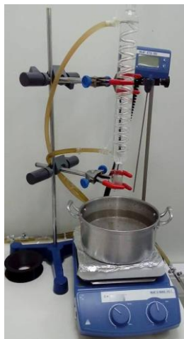
Figure I - Magnetic stirring plate IKA® C-MAG HS 7 with temperature control IKA® ETS-D5.
