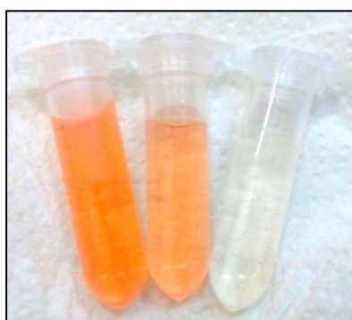
Figure 16 - The samples of supernatants used to analyze drug loading efficiency and drug loading capacity in different pH by UV-Vis at 480 nm (The samples above correspond to pH 6.0, pH 7.4 and pH 8.0, from left to right respectively).
