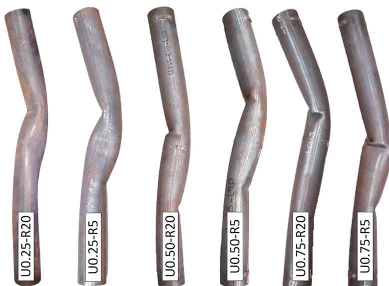
Figura 4.15: Modos de Colapso Experimental das Colunas CHS [3]
