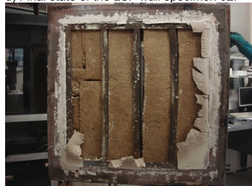
f) Final state of the LSF wall specimen 03.
