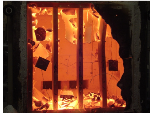
i) average temperature results for specimen 07. j) Final state of the LSF wall specimen 07. Figure 3: Temperature history and limit state for the specimens.
