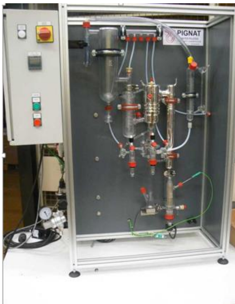
Figure 6. A dynamic recirculation ebulliometer (Societe Pignat, France, modele EEA 3000) [35].
