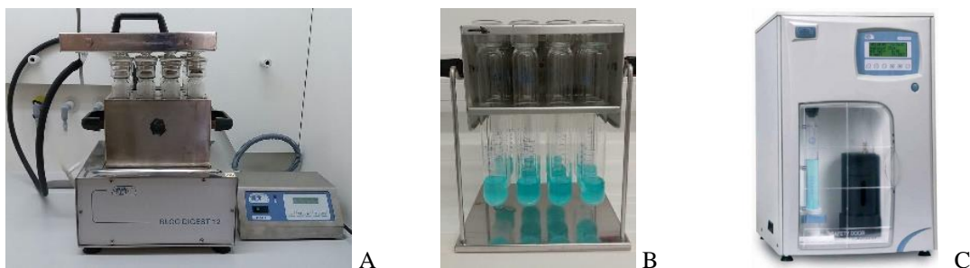
Figure 9. Protein analysis: (A) digester and (B) digested sample quince peel, and (C) automatic distillation and titration unit.
