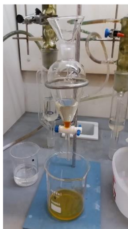
Figure 10. Delipidification step performed with ethyl ether for sugars analysis.
