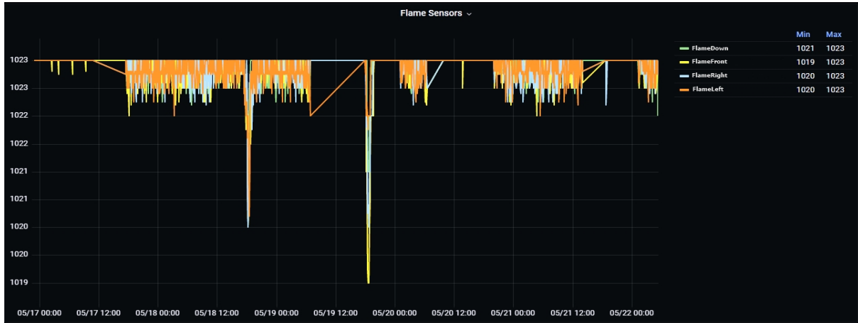
Figure 6.11: Flame Sensors Behavior in Normal Conditions.
