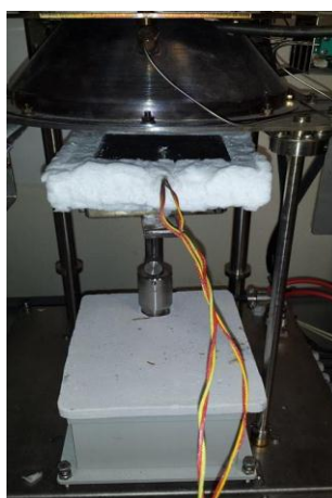
Figure 11: Cone calorimeter and experimental setup.
