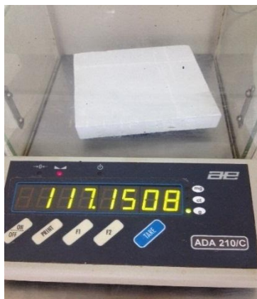
c) Mass before testing of thickness plate dp=15 [mm]
