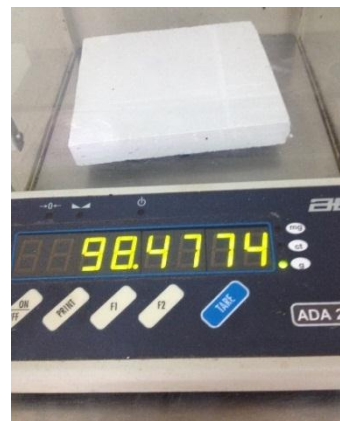
d) Mass after testing of thickness plate dp=15 [mm]
