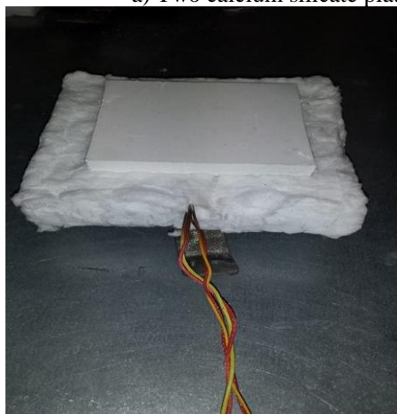
b) Protected carbon steel plate with calcium silicate 15 [mm].
