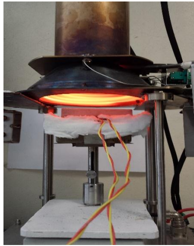
Figure 16: Cone calorimeter and experimental setup.
