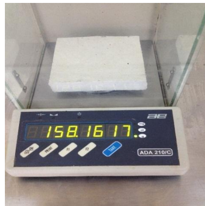
b) Mass after testing of thickness plate dp=20 [mm]
