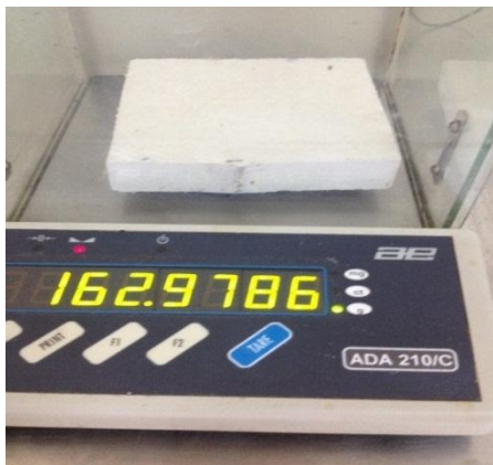
a) Mass before testing of thickness plate dp=20 [mm]
