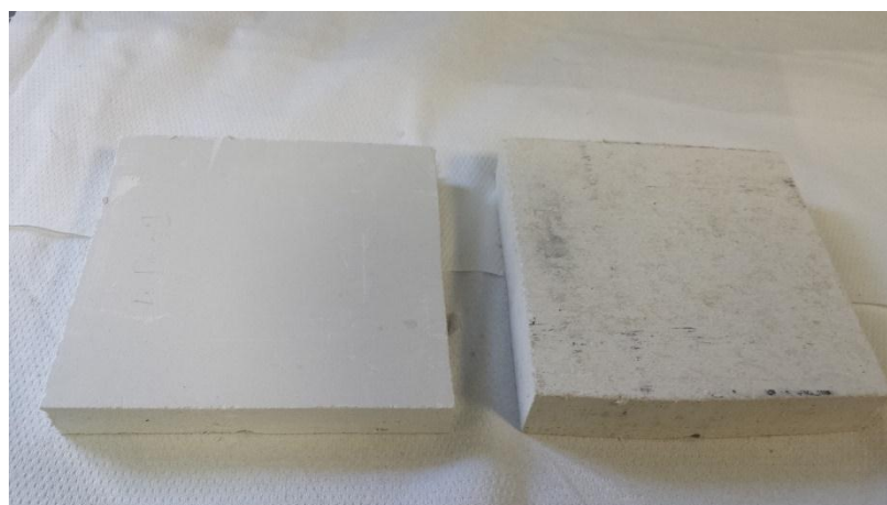
a) Two calcium silicate plates of different thickness: 15 and 20 [mm].
