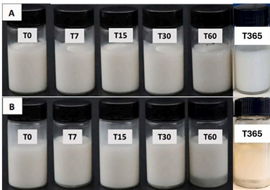
Fig. 8. Macroscopic images of E2 (TM-loaded DPE) during storage at (A) 4 °C and (B) 25 °C over 60 days (0, 7, 15, 30, 60 and 365 days).
