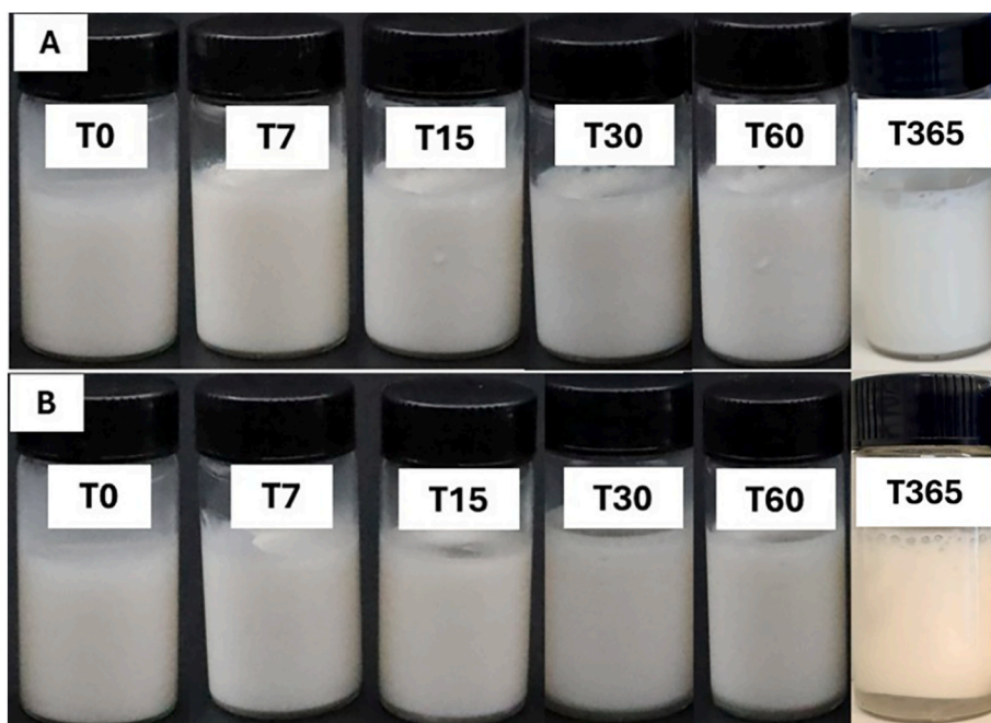
Fig. 7. Macroscopic images of E1 (unloaded DPE) during storage at (A) 4 °C and (B) 25 °C over 365 days (0, 7, 15, 30, 60, and 365 days).
