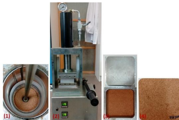
Fig. 1. Experimental system used for the production of cork composites, where (1) mixing the cork with the adhesive, (2) pressing, (3) demolding the composite and (4) cork composite.
