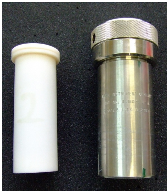
Figure 6.3. View of the autoclave used for hydrothermal synthesis, with PTFE liner.
