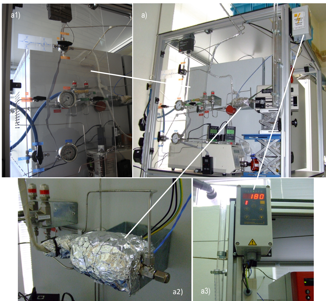
Figure 6.10. Details of the ZEOPERM setup: a1) valves and manometers lateral panel; a2) close-up of the evaporator; a3) close-up of the microprocessor controlled temperature regulator for heat tracing.
