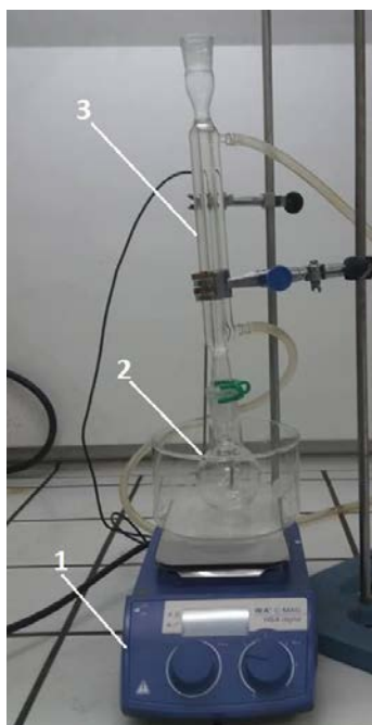
Figure 12. Experimental setup for the esterification: 1) Heater 2) Reactor 3) Condenser.
