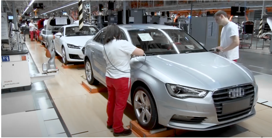
Fig. 3. Measuring gap and flush in the final assembly line (source: https://www.nextsense-worldwide.com/ )
