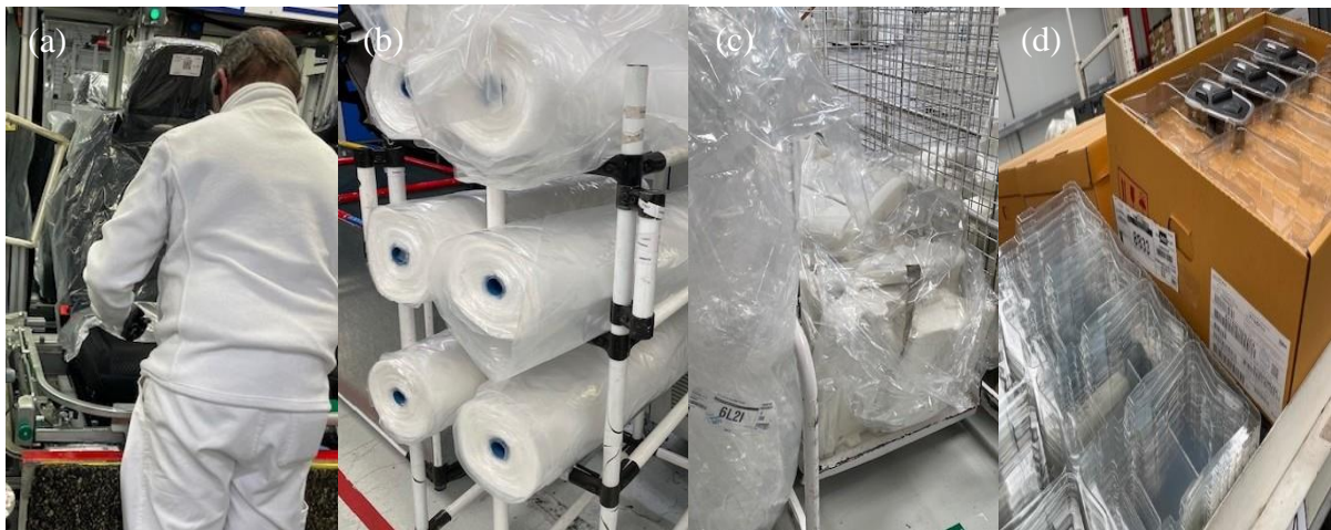
Figure 33 - a, b, c, d. Types of packaging plastic used in the Spanish plants. (a) Rear seat protection cover, (b) LDPE packaging plastic roll, (c) LDPE plastic bag for foams, (d) covers plastic protection
