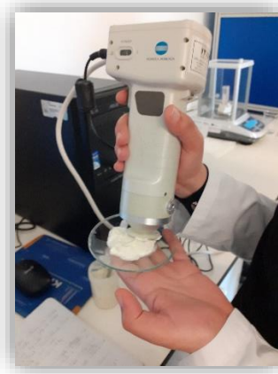
Figure 27: Portable CR400 colorimeter reading a sample
