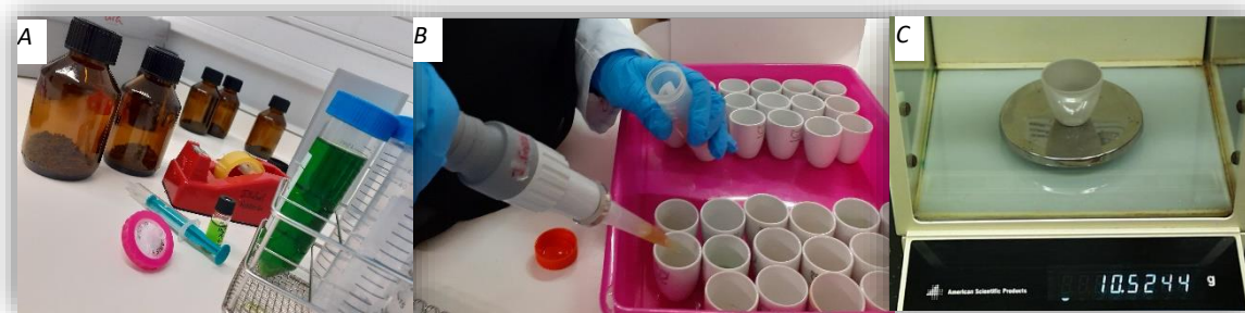
Figure 13: A) Maceration preparation; B) Pipetting to crucibles; C) Weighing the crucibles
