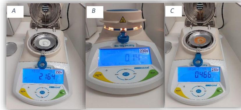
Figure 18: Moisture analysis – A) Weighing 2g of cheese on the balance; B) Evaporation of moisture; C) Final weight
