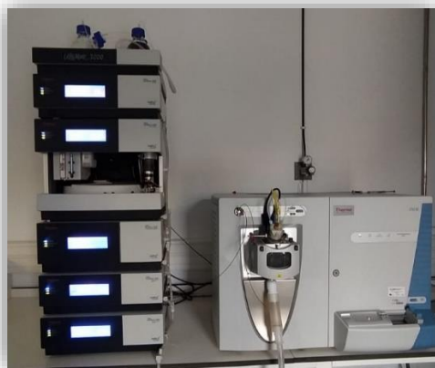
Figure 15: High performance liquid chromatography coupled to diode array detector and to an electro-spray ionization mass detector (LC-DAD-ESI/MSn).
