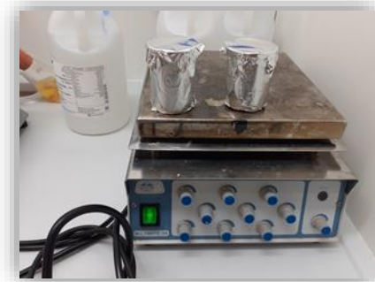
Figure 22: Extraction under magnetic stirring
