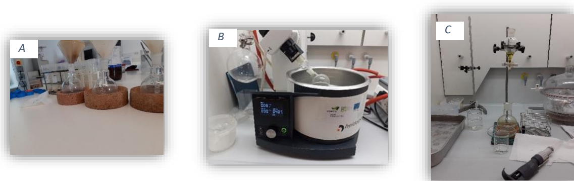
Figure 24: Extraction of soluble sugars – A) Filtration; B) Ethanol evaporation; C) Washing
