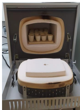
Figure 19: Muffle for sample incineration
