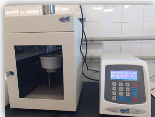
Figure 10: Ultrasonic probe and control device
