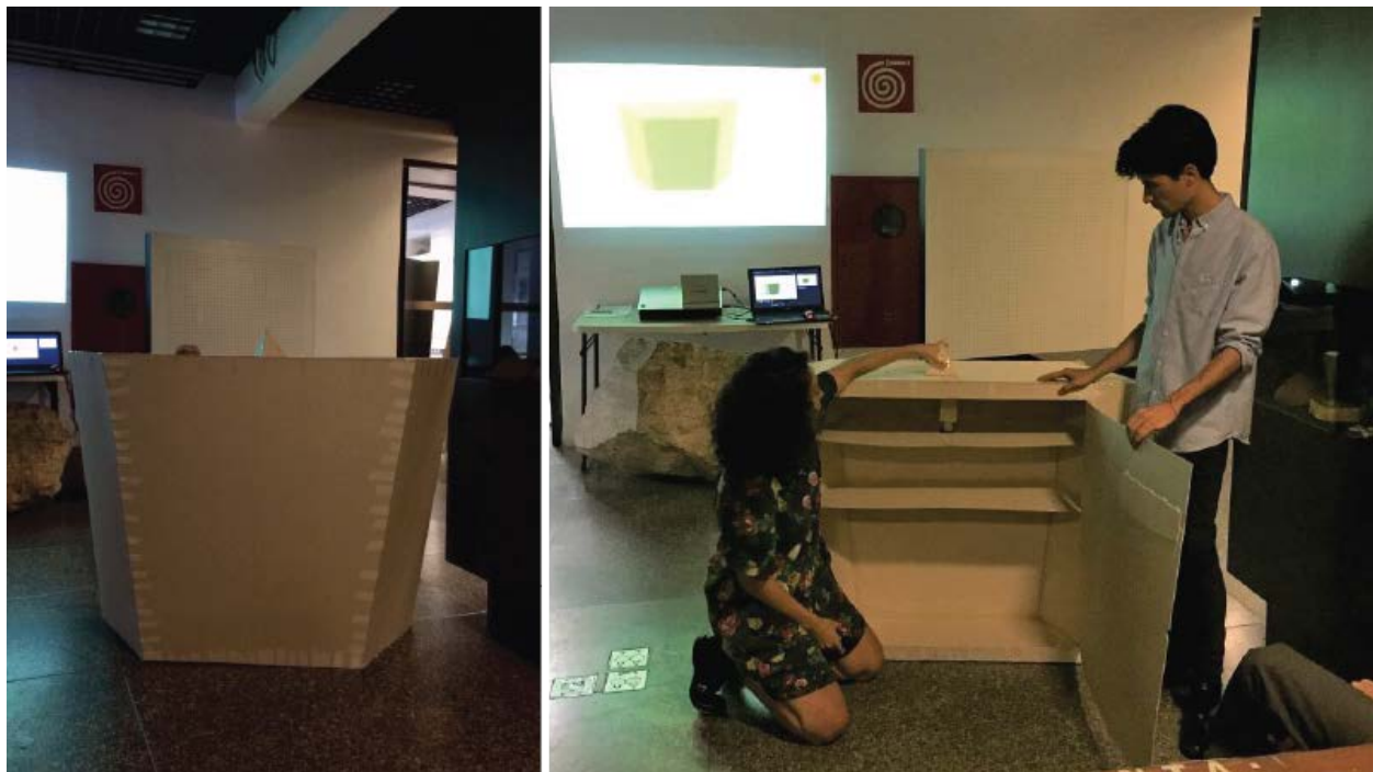
Figure 4: A low-cost prototype of the pilot setup made of cardboard, glue, and adhesive tape (left) and MM Gerda staff and Roberto Vaz presenting it (right). Photos by Roberto Vaz (left) and Ana Cecília Rocha Veiga (right).
