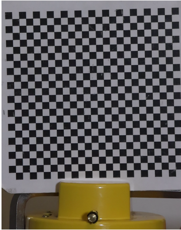
Figure 3.10: A grid pattern with 24 by 23 squares. Each square is 5[mm] × 5[mm] in size.
