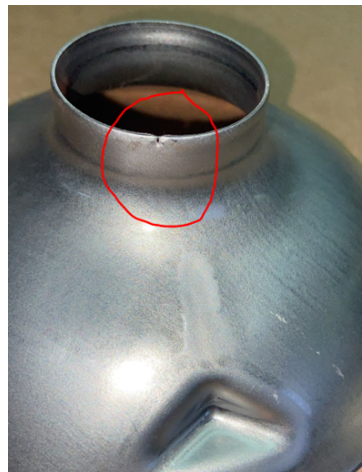
Figure 3.21: Crack in the collar Source: Catraport
