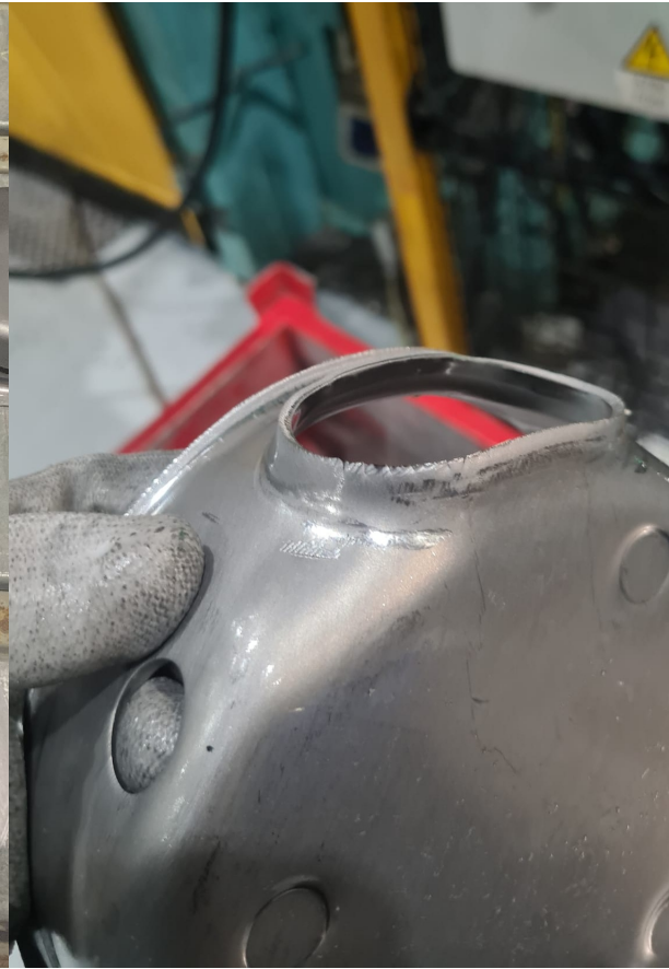
(b) Failure during Collar Formation
