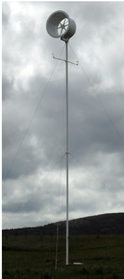
Figure 1.2: Enhanced WT prototype tested at 12 meters in unbuilt environment.
