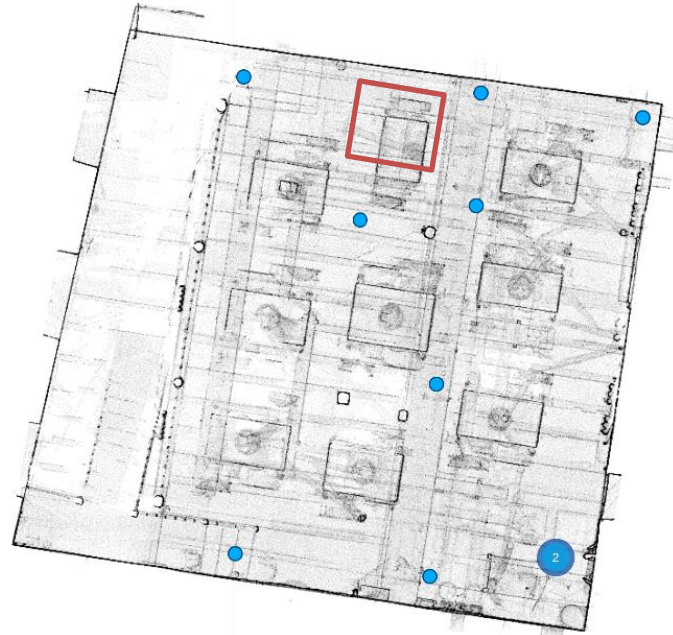
Figure 13: Overview map (red square, machine selected for study, blue points, places where the machine was positioned for the scans)
