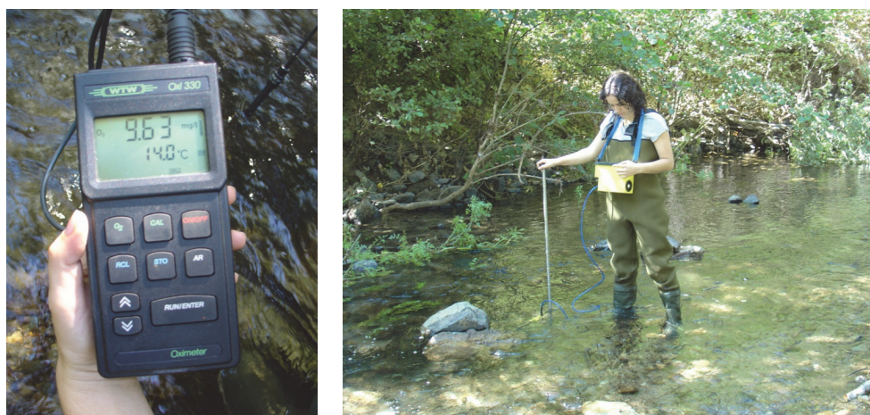
Fig. 4. Measuring temperature (°C) and water column velocity (m.s -1 ) in the Baceiro River (summer 2005).
