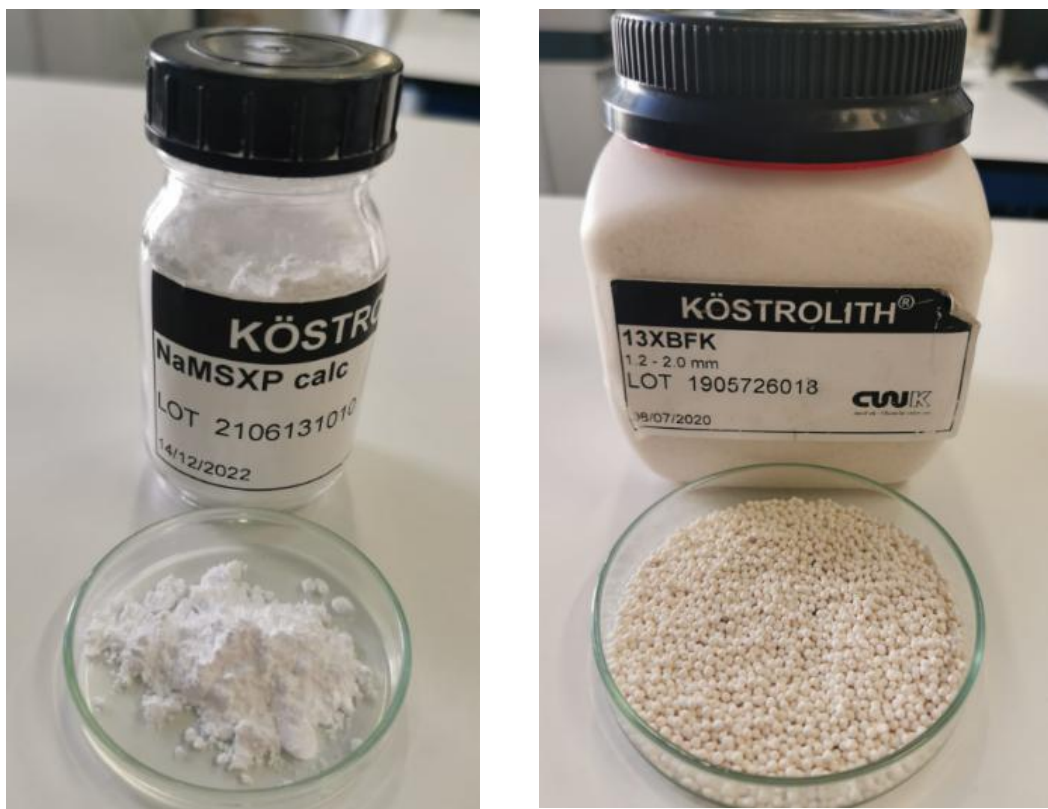
Figure 7. Zeolite 13X powder (left) and beads of binder free (right).
