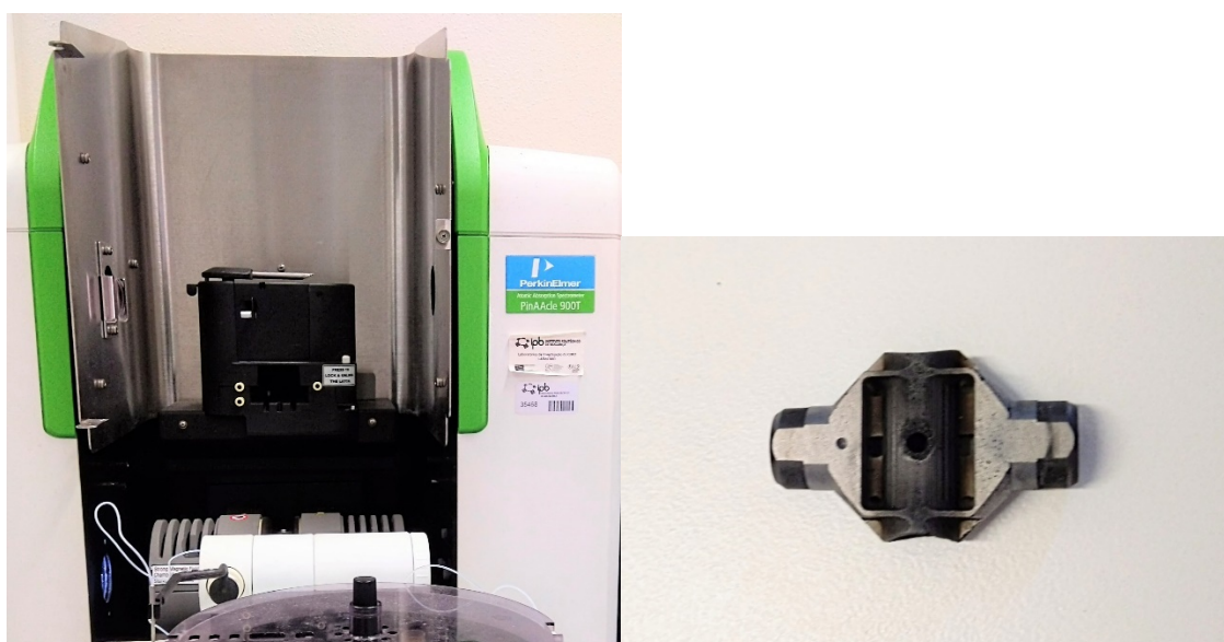
Figure 12. Graphite furnace chamber (left figure) and the graphite tube used (right figure)
