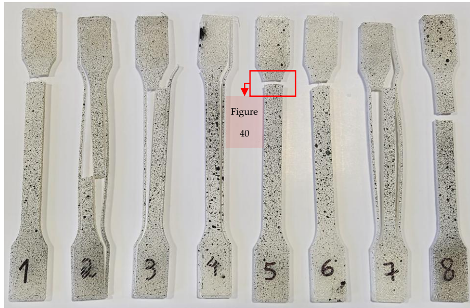
Figure 39. Post-fracture images of representative specimens showing distinct failure locations and profiles.
