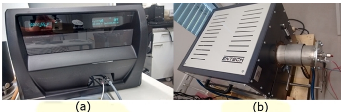
Fig. 2 - Main devices employed. (a) hotdisk equipment and (b) furnace.
