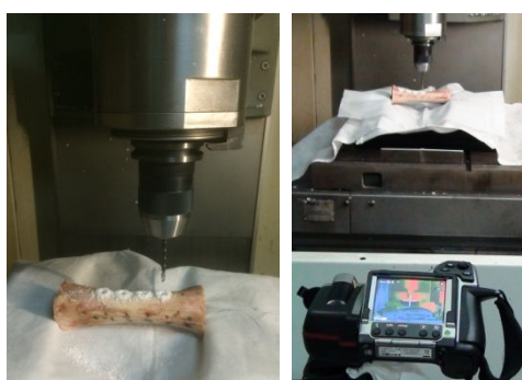
Fig. 5 - Experimental setup: drilling process of bovine bone
