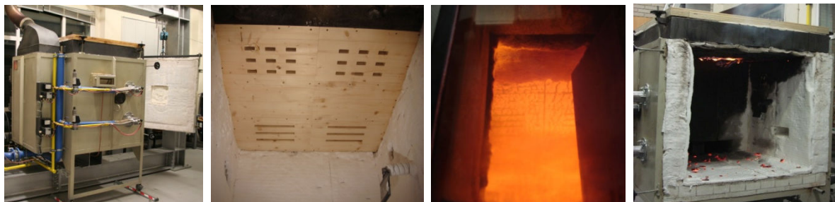
Fig. 6 - Test slab in the fire resistance furnace, before, during and after the test.
