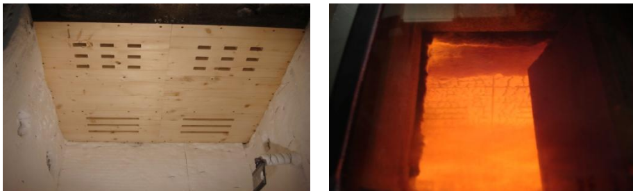
Figure 3: Test slab in the oven, before and during the test.
