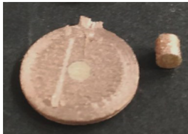
Fig. 1: Broken pin after connector pressure test
