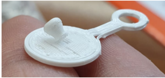
Fig. 4: Broken pin during disconnection
