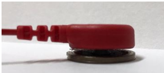
Fig. 5: Gap between electrode's "body" and female snap connector
