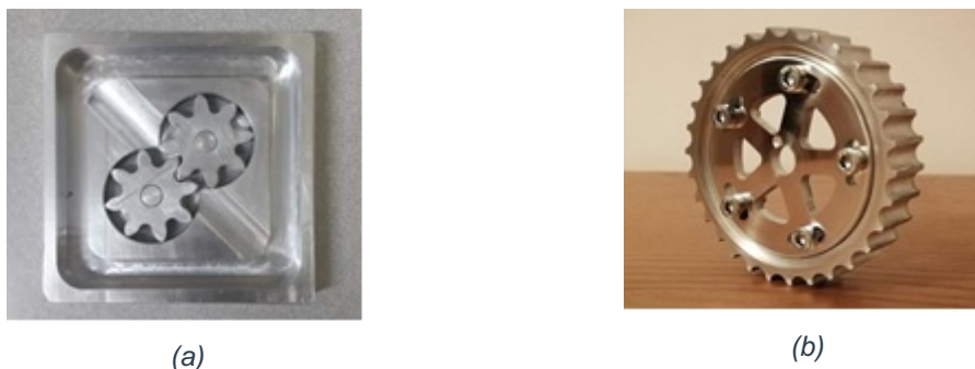
Figure 2. Examples of produced pieces by the students: (a) gear pump and (b) adjustable camshaft sprocket [Source: articles written by students].
