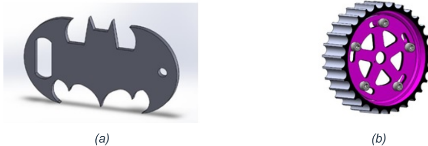
Figure 1. Examples of 3D models design by the students: (a) bottle opener and (b) adjustable camshaft sprocket [Source: articles written by students].
