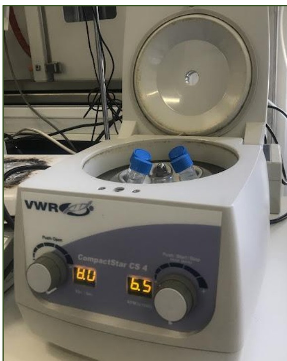
Figure 26: Photographic record of regeneration by centrifugation.
