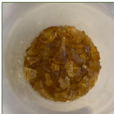
Figure 18: Photographic record of the MIP synthesized considering rutin as template. MIP20.
