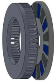
Fig. 1. Single stator-single rotor axial flux machine structure.
